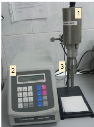
Fig. 1-10. Ultrasonic device consisting of: 1) sonotrode with a titanium tip; 2) ultrasonic processor; and 3) temperature controller.
