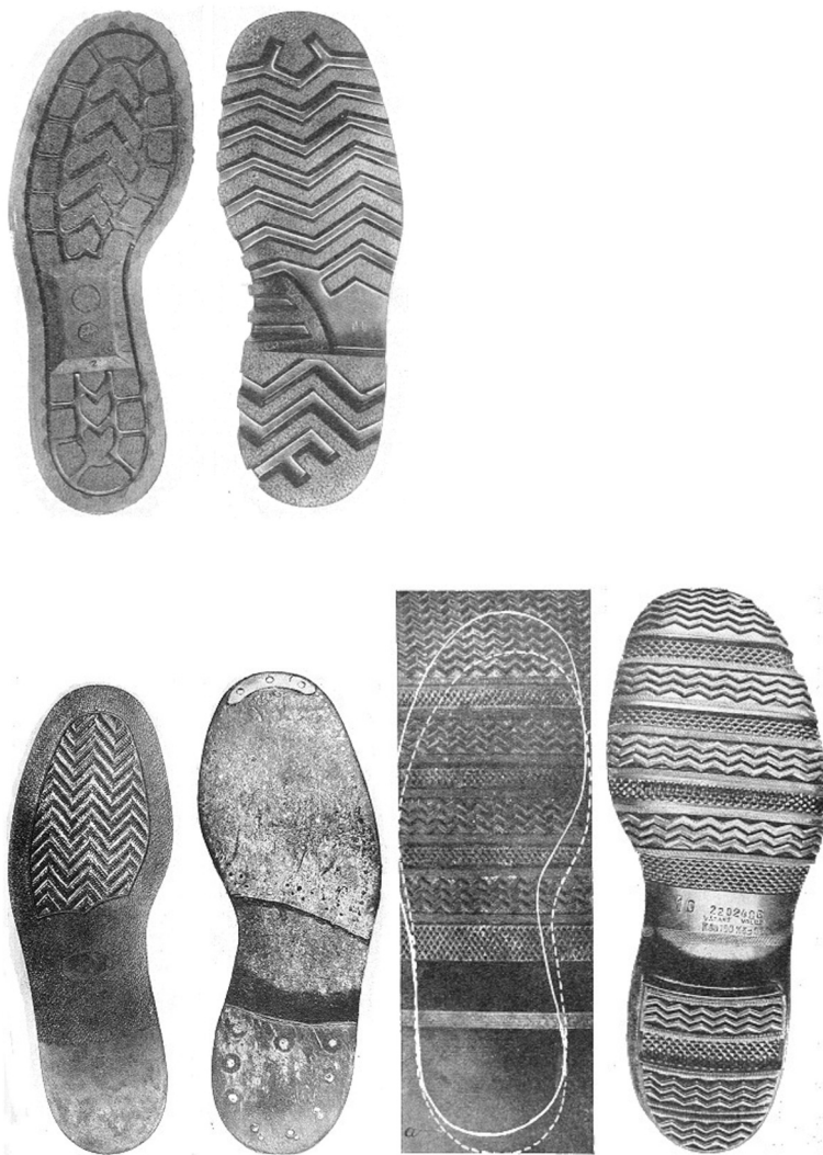
Figure 1-1. Types of soles (monolithic, block sole without heel, doweled with attached sole and heel, part of the rubber plate from which the rolled sole is cut, rolled sole) (Straus, Porada et al, 2004, p. 26-27).
