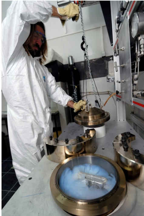
Fig. 2-1. The artist is opening the 20 litter high-temperature supercritical drying reactor after a continuous 48 hours run. The vessel was installed in Greece, September 2005, and all the aer( )sculptures have been created since then in it (photograph and copyright: Massimo Pizzocaro 2/2008).
