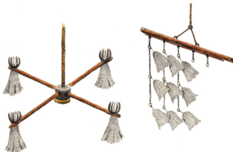
Fig. 1.4 Coral fishing devices: ingegno (left) and Italian bar (right). Reproduced from Cattaneo-Vietti et al. (2017)
