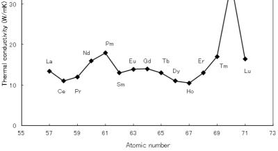
Fig. 1.15 – Values of thermal conductivity of the lanthanides as a parameter of the atomic number in the periodic table
