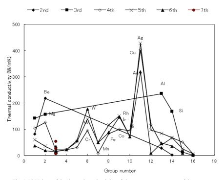
Fig. 1-13 Values of the thermal conductivity of elements as a parameter of the group number in the periodic table
