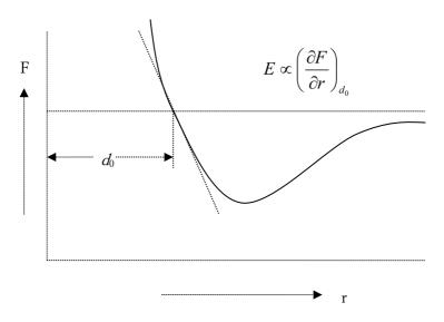
Fig. 1-3 – Interatomic force versus interatomic distance
