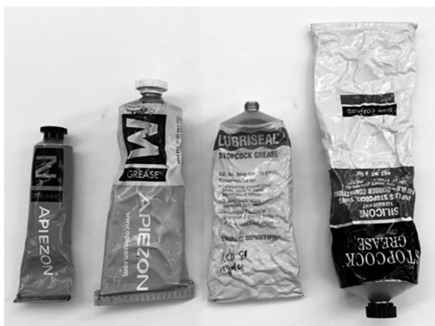
Figure 10. Petroleum-based vacuum greases in aluminum foil tubes.
