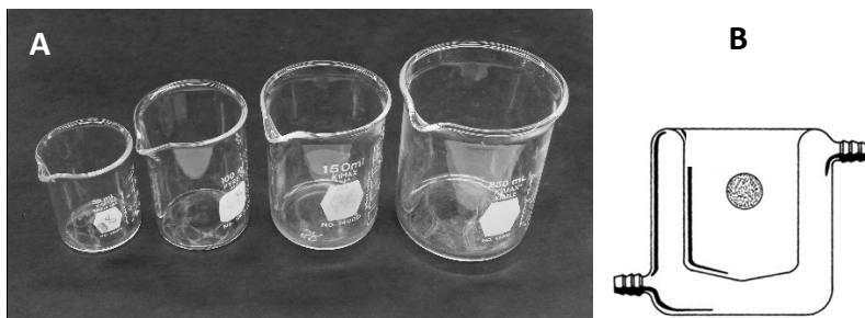
Figure 11. Pyrex beakers of variable sizes (A), and jacketed beaker (B).
