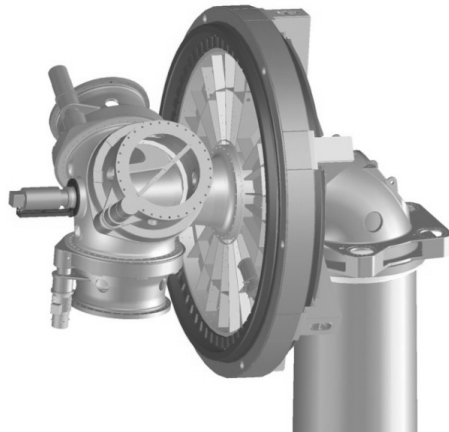
Figure 3. Image of a direct drive of E-48 from Enercon [21]
