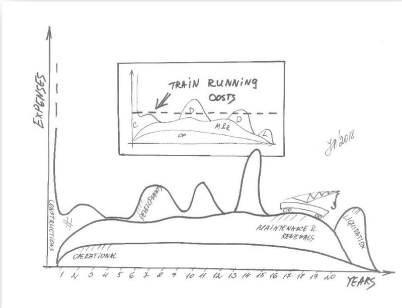
**Figure 1-1.** Costs incurred by train running, based on Beltukov <sup>6</sup>
