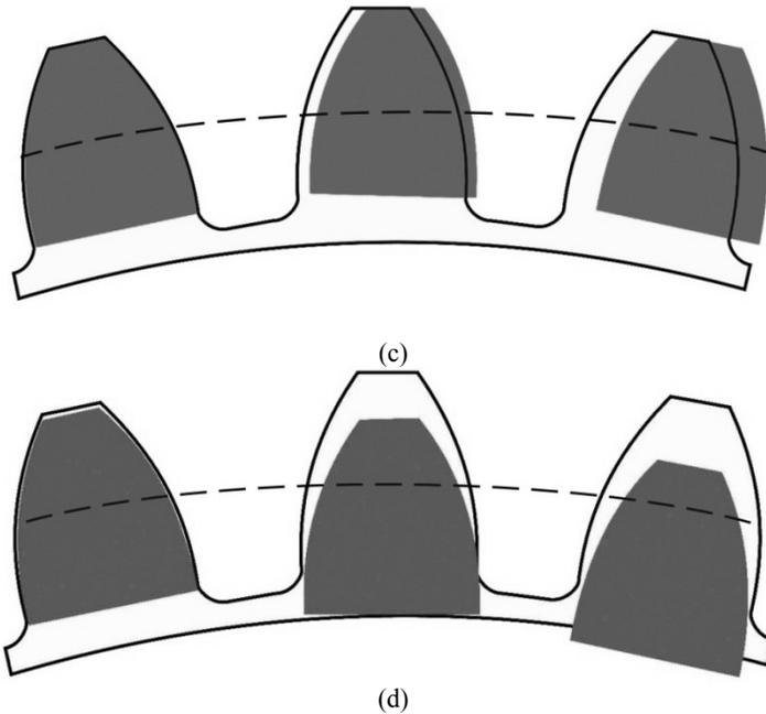
**Fig. 1.4:** Concept of (a) measurement of pitch error and runout; (b) single pitch error; (c) cumulative pitch error; and (d) runout.
