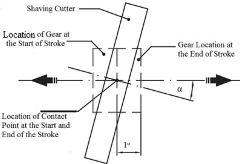
Fig. 1.7: Schematic of transverse gear shaving process.
