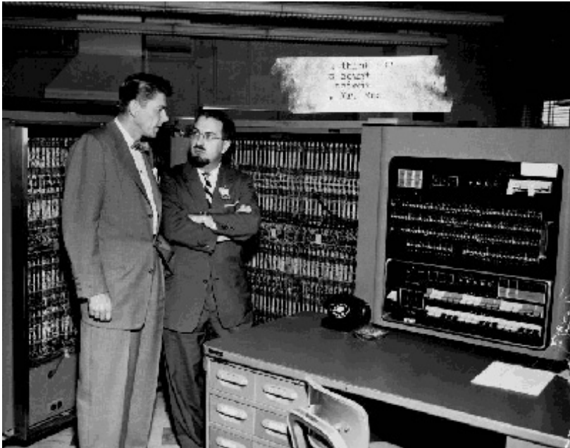
Figure 1-2. IBM 701 at General Electric, Evendale, Ohio Source: Bell 1957
