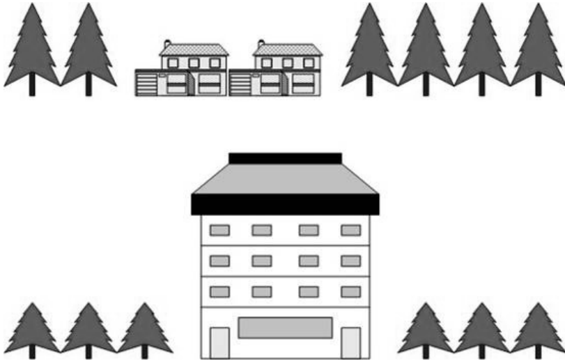
Fig 1.1 Different landscape patterns may appear the same in 2D landscape models due to the missing height information
