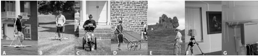
Figure 1-1: Archaeogeophysical Instruments (A) Conductivity Meter, (B) Earth Resistance Meter (C) Ground-penetrating Radar, (D) Optically-pumped Magnetometer (foreground) and Fluxgate Magnetometer (background), (E) Magnetic Susceptibility Meter, (F) Time of Flight 3D Laser Scanner, and (G) Laser Triangulation 3D scanner.
