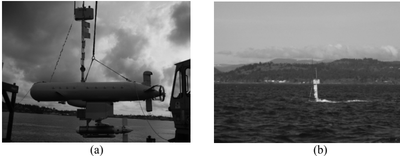
Figure 1: The semi-submersible remote minehunting vehicle DORADO (a) out of the water (b) underway
